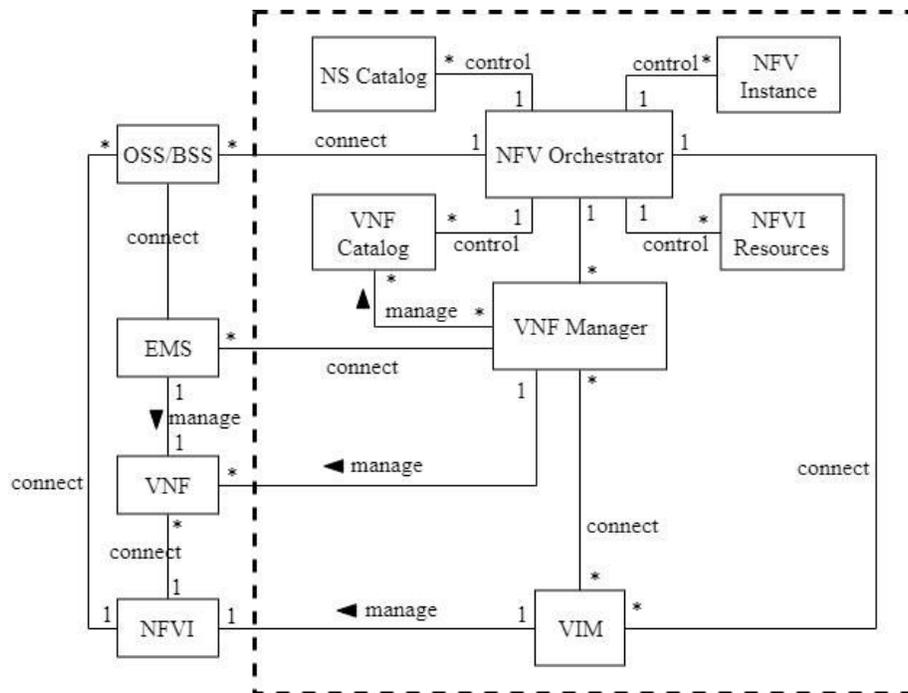
Figure 2. Class diagram for the structure of MANO unit
