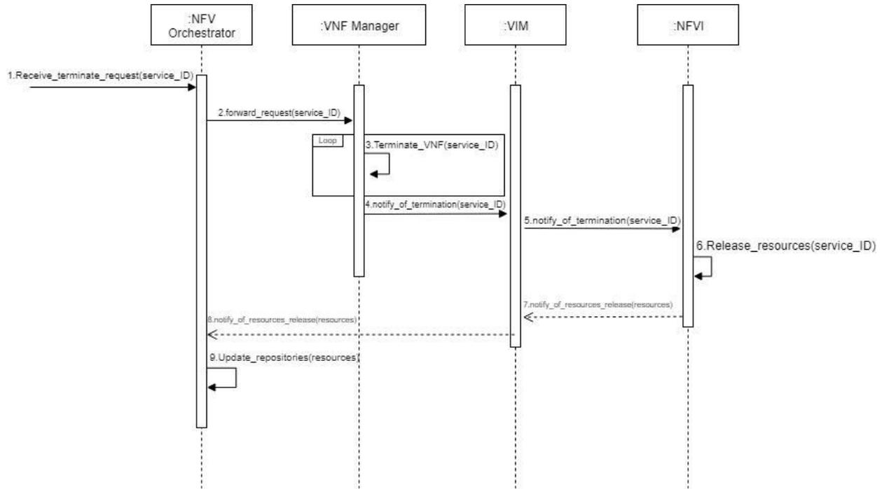
Figure 4. Sequence diagram for service termination.
