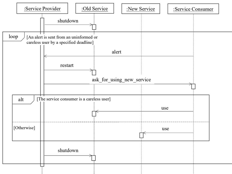
Figure 3. Sequence diagram of the Shutdown-Alert pattern.
